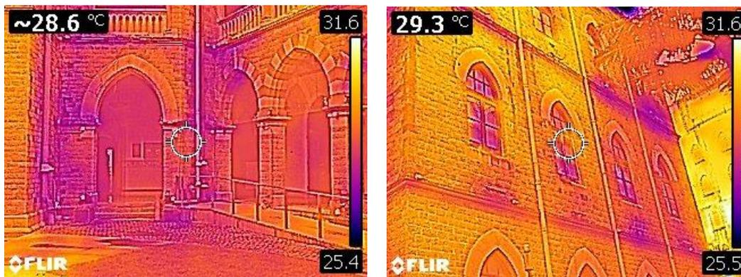
Figure 2 & 3: Thermal images of the façade from the inner courtyard, Source: Author
