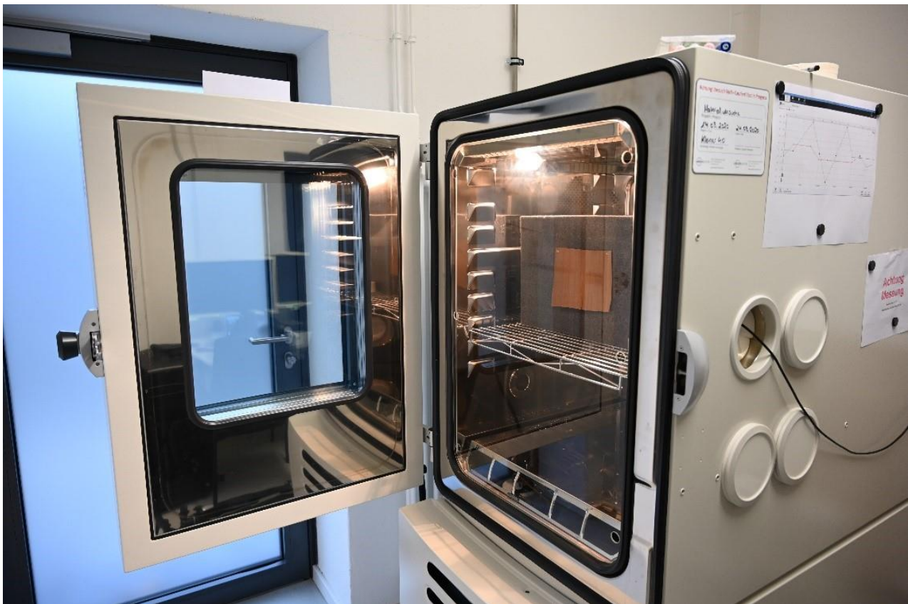
Fig. 1. Climate test chamber ClimeEvent C/340/40/3/M from Weiss Umwelttechnik GmbH with the wood veneer inside. (© Anne Karl, KDWT University of Bamberg).
