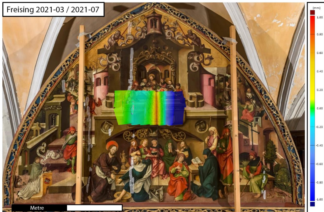
Fig. 1. The wooden panel painting of Freising with the overlay of the superimposed false colour image shows the deviation between the two SLS-Scans from March 2021 and July 2021. Movements of approximately \pm 1.0 mm can be seen. Red meaning a convex warping and blue meaning a concave warping (© Leander Pallas).
