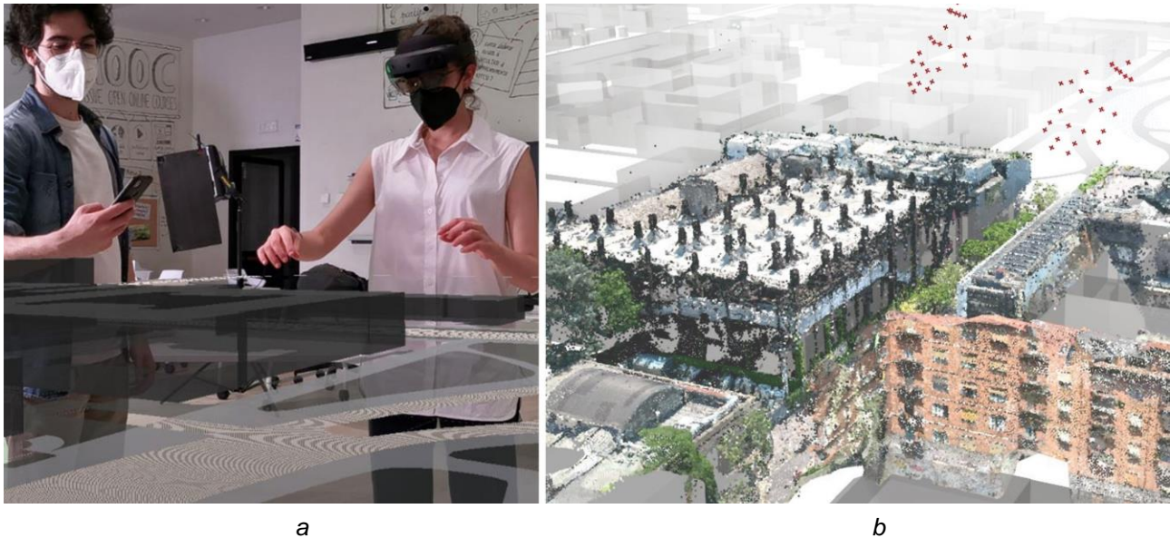
Fig. 1. Mixed Reality simulation on a brutalist Cultural Heritage building: the Fologram app on HoloLens 2, iOS and Android. a) users with smartphones and AR headsets interact with a b) 3D model and a point cloud in Rhino.
