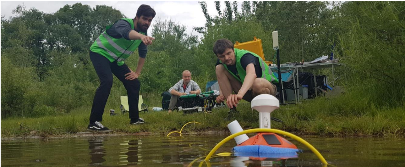
Fig. 3. This photo shows the buoy during its first test deployment in the Oberwartha reservoir. The large white L5 GPS antenna at the top of the buoy and the smaller white wireless LAN antenna at the side are well visible. Furthermore, here is the additionally attached blue buoyancy body which is necessary because of the additional weight. Conclusion and Future work
