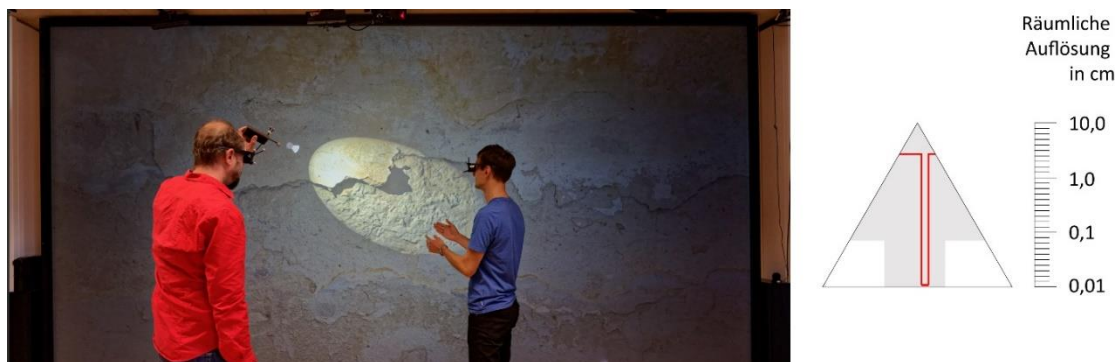
Figure 1: Virtual illumination of a detail scan with submillimeter accuracy ((C) Bauhaus-Universität Weimar) For particularly interesting areas, models were created with sub-millimeter precision. Since this resolution is not available for the entire model, the pyramid is not completely filled in the lower area. For each new perspective on the data, only a small section is needed. This section through the data is illustrated here in a highly simplified way as a red line. [Kulik et al., 2018]
