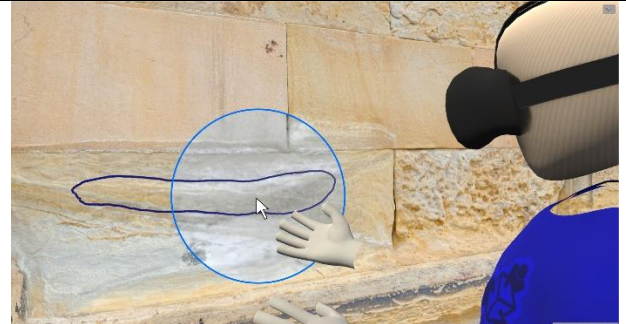
Figure 3: A detail of Hummelshain castle with an overlay of the reflexion coefficients of a registered laser scan in a lens ((C) Bauhaus-Universität Weimar)
