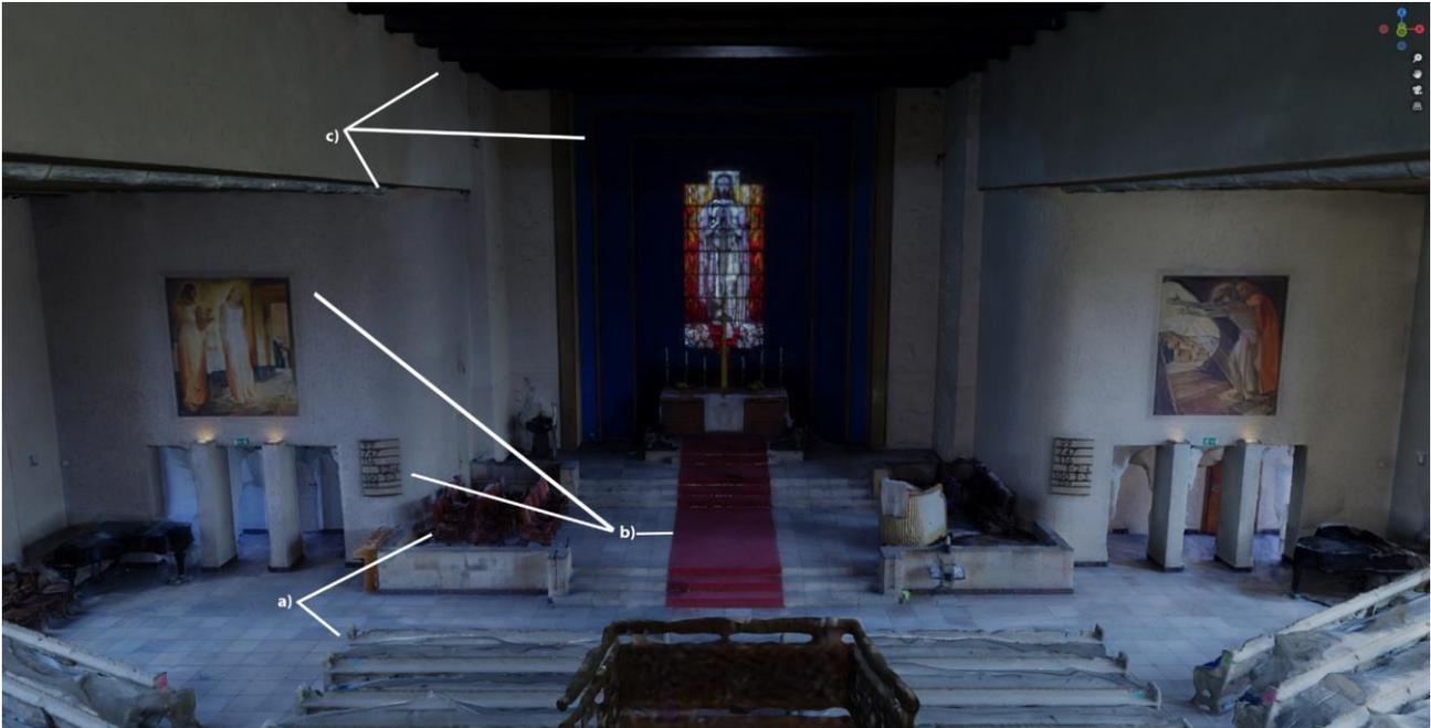
Fig. 1. Photogrammetric 3D model of the interior of a church in Leipzig with different object classifications, a) repetitive objects (chairs & benches); b) different surface structures (painting, plastic and carpet); c) special geometrical features.
