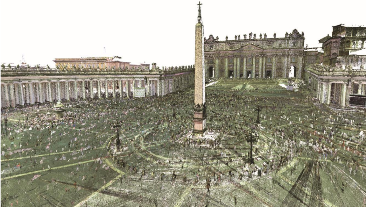
Fig. 1. 1 San Pietro's Square, view of the numerical model resulting from the processing of data acquired by 3D laser scanning.
