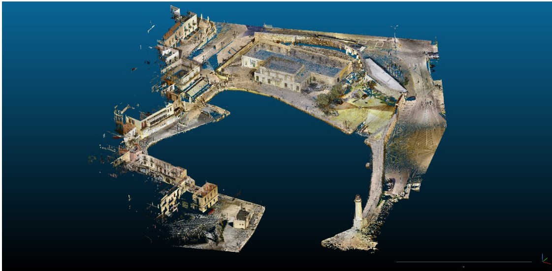
Fig 2. Isometric view of the pointcloud derived from integration of TLS and RPAS photogrammetry.
